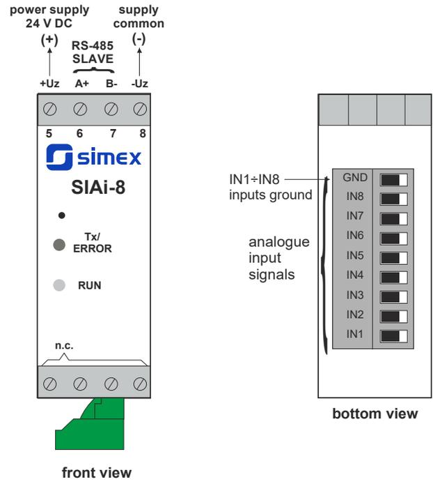
Connection and principle of operation
