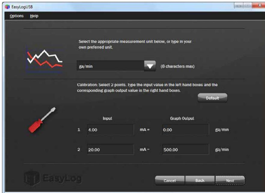
Select the calibration for your data logger. The data logger will always measure current in the 4 to 20 mA range. If you selected Custom Calibration, then the 4 to 20mA measurement range of the EL-USB-4 will be translated into a graph scale of your own choice, with a unit name of up to 8 characters long (e.g. m/s, gal/min, mA, etc.).
