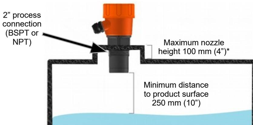
\* Please note that nozzle heights exceeding this value may disrupt the transmitted signal and interfere with level measurement.
